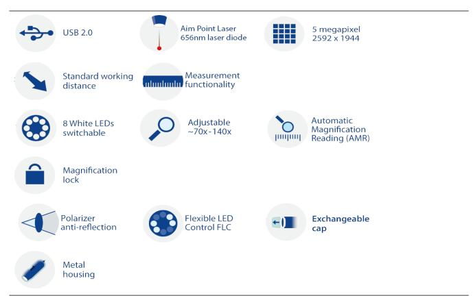
The AM7515MZT1P is part of the universal range and with its standard working distance and wide magnification range from 70-140x, it is suitable for a wide range of applications. Because of the built-in polarization filter this model is ideal when working with shiny or reflective objects such as metal, plastic, glass, jewelry, electronics, etc. The AMR function is of particular importance when the measurement functions are frequently used.
